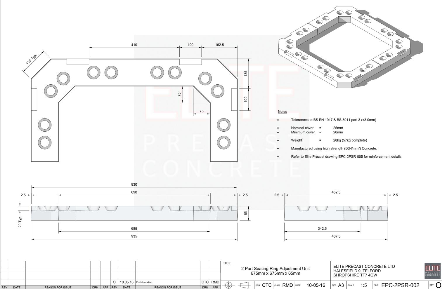
EPC-2PSR-002\_O - 2 Part Seating Ring Adjusting Unit - 675mm x 675mm x 65mm
