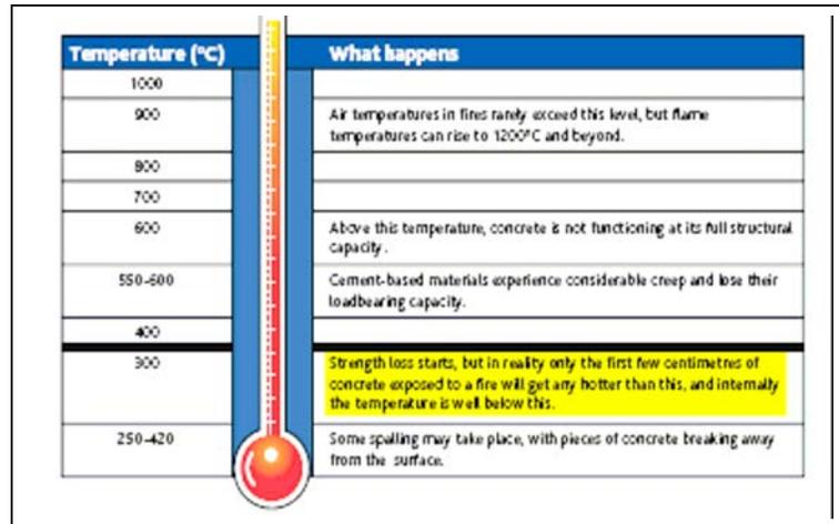
**Figure 2.1:** Concrete in fire: physical processes. (Khoury 2000)
