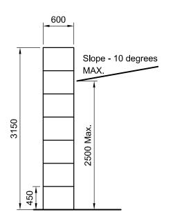
Important Note - The retained material should be allowed to naturally fall against the wall as it is stacked. Do not allow the retained material to stand up on its own as this could lead to a catastrophic failure of the material and the wall.
