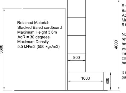
Retained Material:-Baled cardboard AoR = 30 degrees Maximum Density 5.5 kN/m3 (550 kgs/m3)
