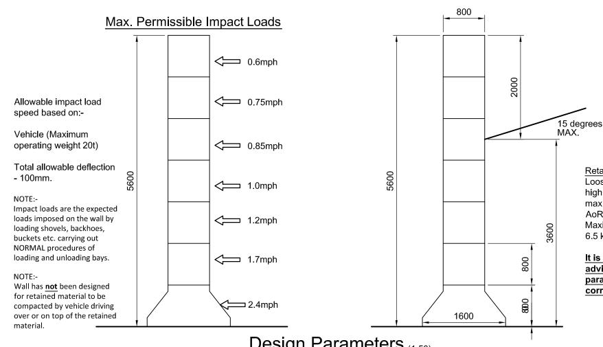
Retained Material:-Loose wood up to 3.6m high and sloped at a maximum of 15 degrees. AoR = 25 degrees Maximum Density 6.5 kN/m3 (650 kgs/m3)
