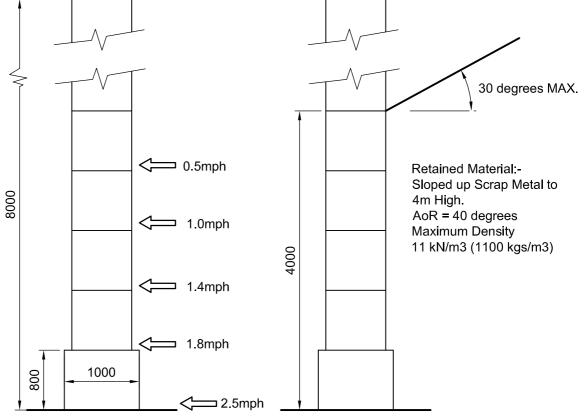
Allowable impact load speed based on a total deflection of 150mm and a vehicle weight of 20t
