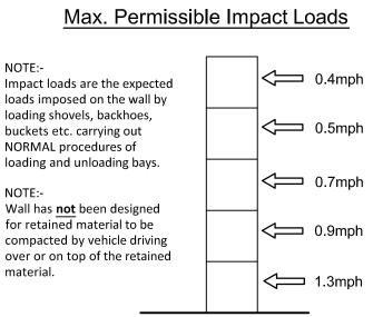
Allowable impact load speed based on a total deflection of 100mm and a vehicle weight of 20t
