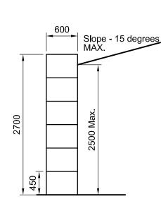
Important Note - The retained material should be allowed to naturally fall against the wall as it is stacked. Do not allow the retained material to stand up on its own as this could lead to a catastrophic failure of the material and the wall.
