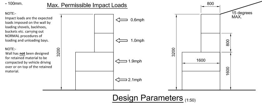
Important Note - The retained material should be allowed to naturally fall against the wall as it is stacked. Do not allow the retained material to stand up on its own as this could lead to a catastrophic failure of the material and the wall.
