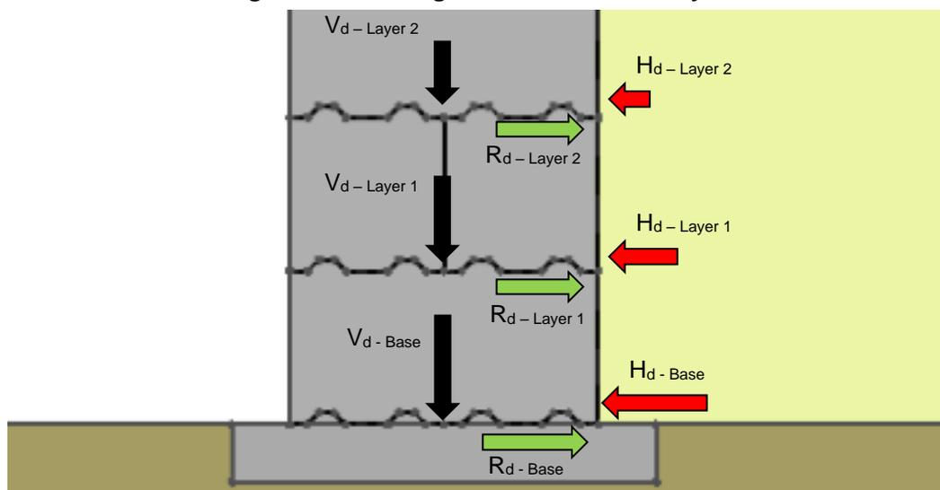
The horizontal design action,  $H_d$ , is the total horizontal force applied at the base of each block. It comprises the retained earth pressures due to self-weight of the backfill and vertical surcharge, plus any additional horizontal actions such as impact loads.
