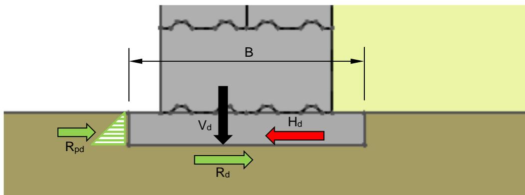
The horizontal design action,  $H_d$ , is the total horizontal force applied at the base of the foundation. It comprises the retained earth pressures due to self-weight of the backfill and vertical surcharge, plus any additional horizontal actions such as impact loads.
