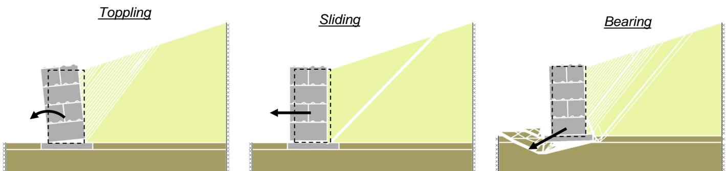
The retained ground (or stored materials) and imposed surcharge loads exert pressures on the retained side of the wall (see Figure 2.2). These are considered ‘unfavourable’ actions as they are acting to de-stabilise the structure. The self-weight of the retaining wall is usually a ‘favourable’ action, as the effects of it are to counter the effects of the unfavourable actions. For bearing failure, the self-weight of the wall may be ‘favourable’ or ‘unfavourable’.
