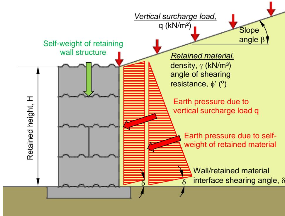
Methods for determining the values of retained earth pressures are included in Annex C of Eurocode 7. For gravity walls at the ultimate limit state, it is assumed that sufficient wall movement has occurred for active conditions to be applicable. The retained earth pressure,  $\sigma_a$ , is then calculated using the active earth pressure coefficient,  $K_a$ , based upon expression C.1 in Eurocode 7:
