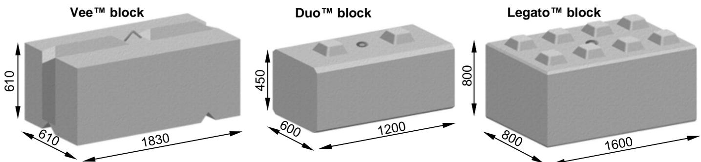
These interlocking block systems may be used for both free-standing walls and retaining walls. Typical free-standing wall applications include:
