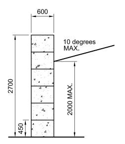
Retained Material:-Lightweight Material AoR = 35 degrees Maximum Density 10 kN/m3 (1000 kgs/m3)
