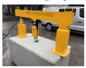
Legato Block at 50% loading of 5.0t Pin Anchor
