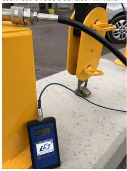
200% load on Duo Block 2.5t Pin Anchor
