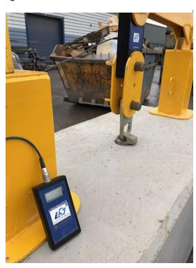
Checking depth of Pin Anchor Head.
