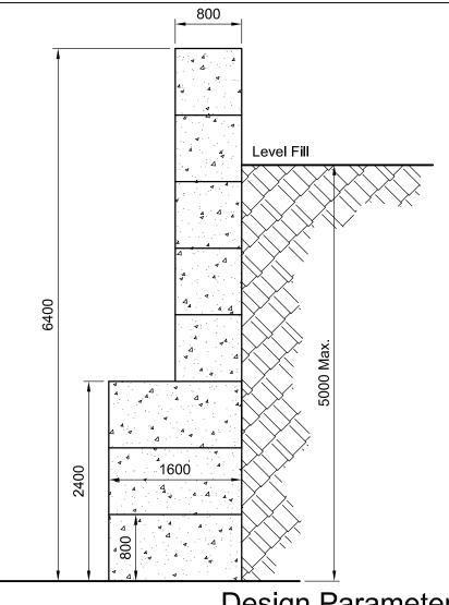
Important Note - The retained material should be allowed to naturally fall against the wall as it is stacked. Do not allow the retained material to stand up on its own as this could lead to a catastrophic failure of the material and the wall.
