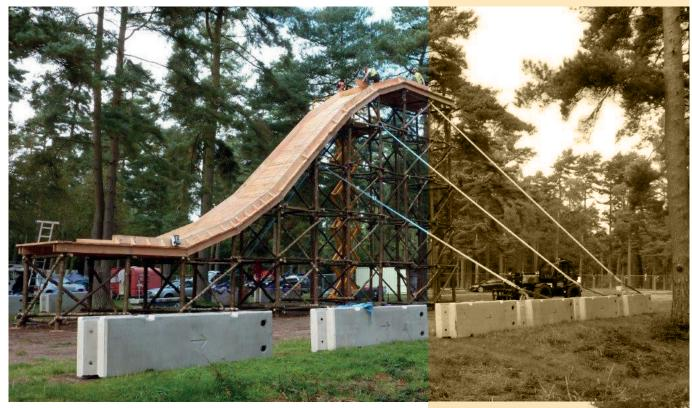
A clay model of a Rover 75, the last car produced at the Longbridge works nearby, was lifted onto the 10 metre high ramp by crane. Then the 1.5 ton car was made to freefall down the ramp and crash into the TVCB concrete safety barriers at the end of the safety zone.
