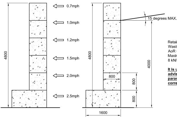
Retained Material:-Waste to 4m High. AoR = 35 degrees Maximum Density 8 kN/m3 (800 kgs/m3)
