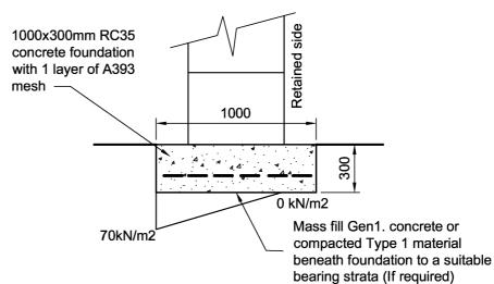
**Bearing Pressure Directly Beneath Wall**
