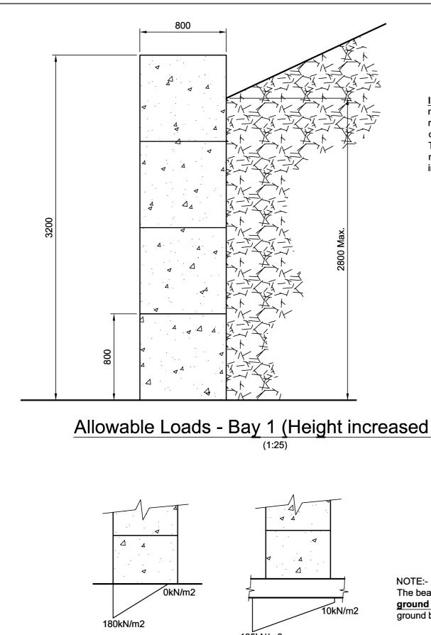
Important Note - The retained material should be allowed to naturally fall against the wall as it is stacked. Do not allow the retained material to stand up on its own as this could lead to a catastrophic failure of the material and the wall. The wall has not been designed to withstand the impact of the retained material suddenly falling against the wall due to incorrect loading.
