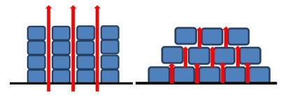
Far left: Standard bale storage may result in chimneys between bales promoting air-flow during a fire. Left: Interlacing bales may disrupt this chimney effect reducing air-flow and fire intensity
