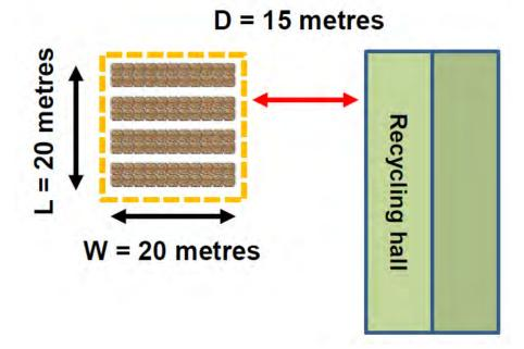
Limited space at this site means the maximum separation distance which can be achieved between recycling building and stack is 15 metres (D in graphic). Using paper/card bales as for example B above, graph 1 purple line gives a maximum stack length of 20 metres (mark 15 metres on the vertical axis of graph 1, draw a horizontal line across to the purple line, and then a vertical line down, giving stack length at some 20 metres). This is an example of a reverse use of the data in graphs 1 and 2.
