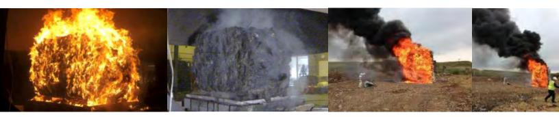
From left: HDPE bale burn during phase 1 smaller scale tests, and same post-burn showing relatively intact bale. Compared to larger scale simulated plastics waste bale stack burns
