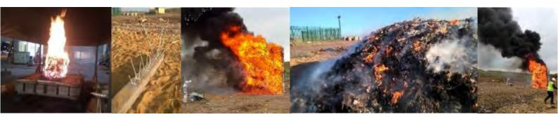
General views WISH fire tests, from left: Smaller scale laboratory burn tests, the 'porcupine' thermal sensor array used in larger scale stack burns, plastic bales burn test, RDF loose stack burn test, bale burn test general view.
