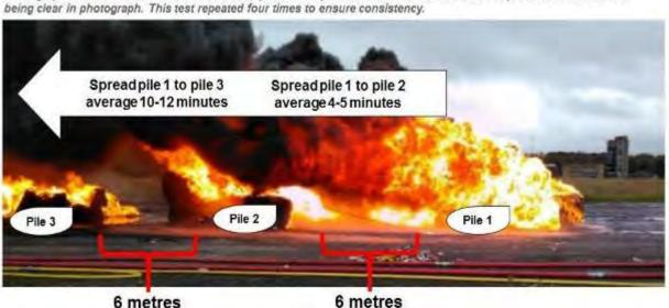
Photograph of actual tests. Note, bale stacks in partial collapse and extensive flames result in pre-burn distances not
