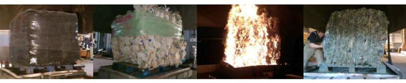
From left: Baled RDF pre-burn, baled LDPE plastic pre-burn, during burn and post-burn (note bale post-burn showing relative lack of fire penetration leaving the bale largely unburnt)
