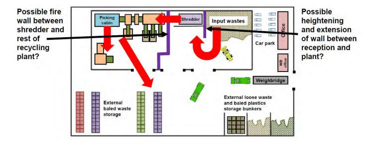
While this would not split the building into 'true' compartments, consideration could also be given to raising the height of and extending the length of the push-wall between waste reception and the shredder to reduce the risk of fire spread (see below on fire walls at bunkers etc).
