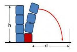
Example of a stack collapse mechanism, assuming a bale at the base of the stack collapses first. The distance any bale, or part of a bale, will 'roll' is dependent on a range of factors making stack collapse too unpredictable to use as a guide to separation distances between stacks
