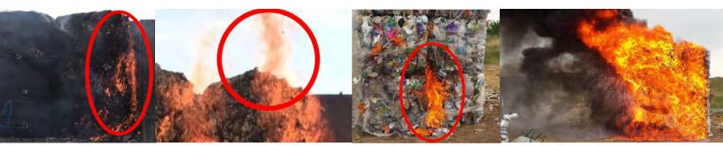
From left: Development of fire vortex behaviour during bale burn tests, visible fire vortex at top of gap between bales during bale tests, development of fire spread in gaps between bales, leading rapidly to a fully developed fire (see bale comments above)
