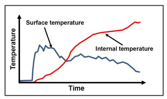
Graph 2: Phase 1 illustrative loose pre-crush wood internal and surface temperatures
