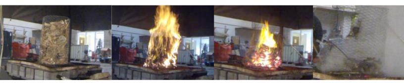
From left: Loose pre-crush wood waste pre-burn (note retained in mesh 'cage'), in initial phases of burn, during steady state burn and post-burn (note much more complete combustion than for baled wastes)
