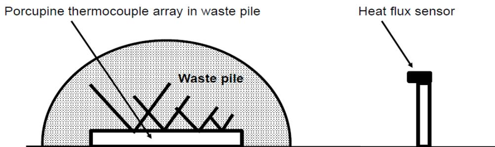
Ignition for surface (outside-in) burns was via use of a 'blow-torch', or in some cases for bales domestic fire-lighters. Ignition for deep (inside-out) burns was via domestic fire-lighters introduced to the centre of piles. Unlike the smaller scale phase 1 tests, wastes were allowed to 'burn-out', with the exception of loose plastics, which emitted large volumes of black smoke and was extinguished before burn-out occurred.
