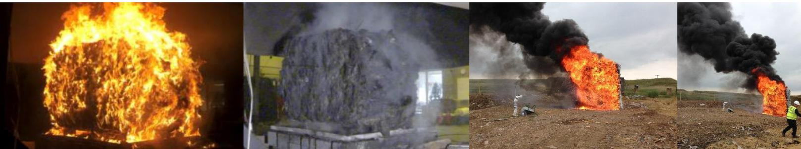
From left: HDPE bale burn during phase 1 smaller scale tests, and same post-burn showing relatively intact bale. Compared to larger scale simulated plastics waste bale stack burns
