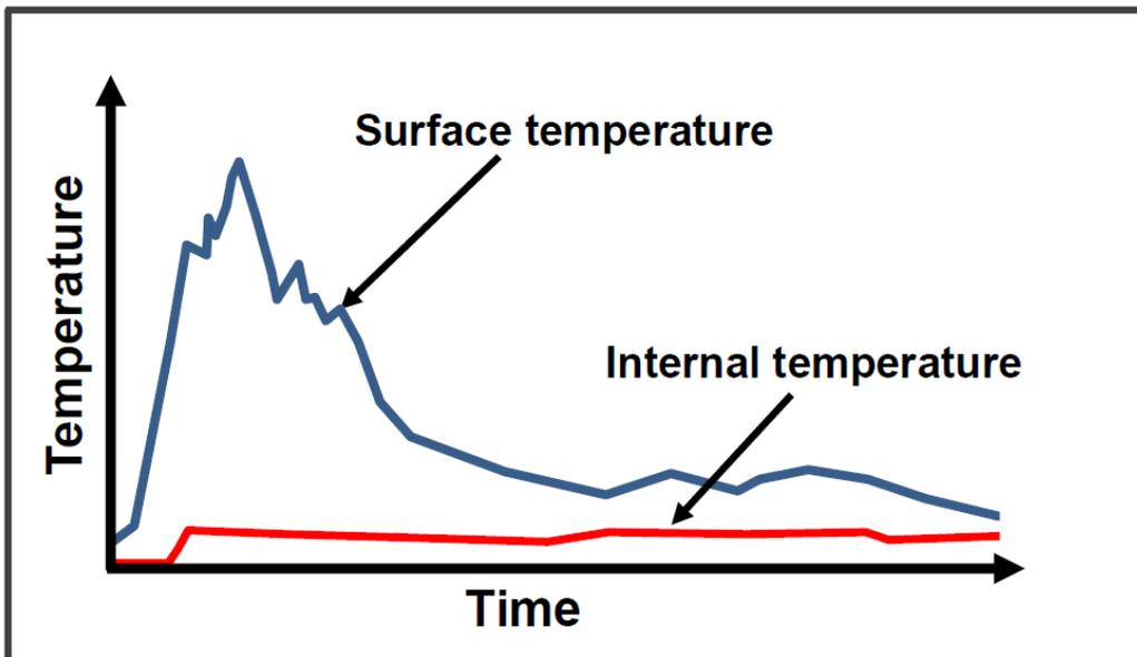
Also as for baled wastes a 'char' layer formed at the surface of the pile on most of the larger loose waste storage piles, restricting fire penetration, and resulting in a more prolonged 'smouldering' type burn once the initial phase of burn had declined. This pattern replicates more closely typical FRS experience when tackling some loose waste pile fires.
