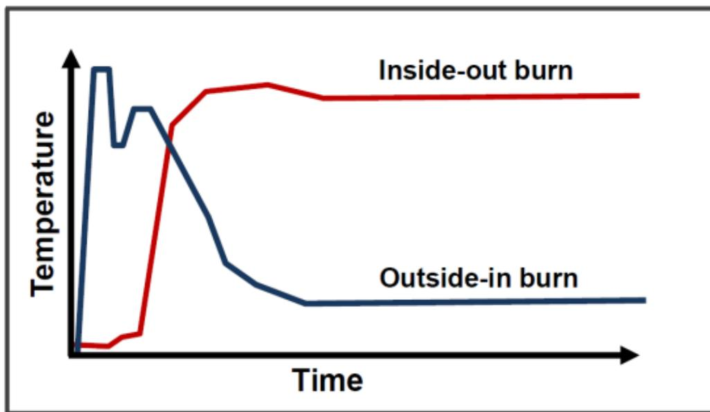
During inside-out burn tests fires took longer to develop. Probes within the loose waste stacks (the 'porcupine') show the build-up of a 'super-heated' bed within the waste stack. This slowly burns outwards, and then breaches the surface as a fully-developed and energetic fire. This inside-out mechanism results in sustained higher temperatures, rather than the dying-back of temperatures observed during loose waste stack outside-in fires.
