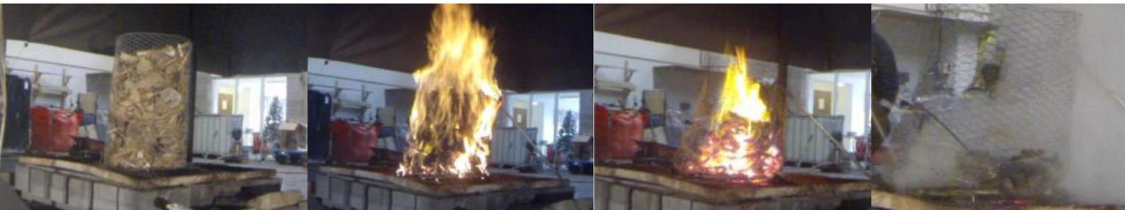
*From left: Loose pre-crush wood waste pre-burn (note retained in mesh 'cage'), in initial phases of burn, during steady state burn and post-burn (note much more complete combustion than for baled wastes)*
