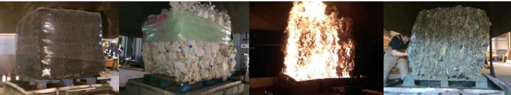
*From left: Baled RDF pre-burn, baled LDPE plastic pre-burn, during burn and post-burn (note bale post-burn showing relative lack of fire penetration leaving the bale largely unburnt)*
