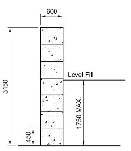
Important Note - The retained material should be allowed to naturally fall against the wall as it is stacked. Do not allow the retained material to stand up on its own as this could lead to a catastrophic failure of the material and the wall.
