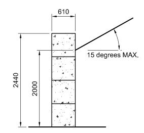
Retained Material:-Wheat to 2m High. AoR = 27 degrees Maximum Density 7.5 kN/m3 (750 kgs/m3)
