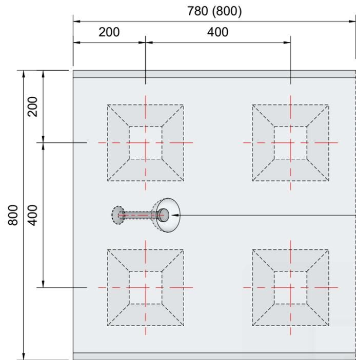
Ø94mm dia semi-spherical recess in gravitational centre of block for pin anchor.
