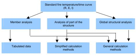
Figure 3.3: Design procedure for fire resistance of structures
