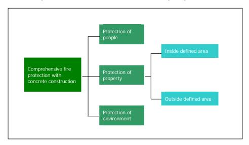
Figure 1.1: The comprehensive approach to fire safety (Courtesy Neck, 2002)
