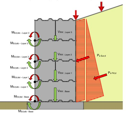
Figure 4.2.3 Toppling resistance of each layer of blocks
