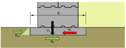
The horizontal design action,  $H_d$ , is the total horizontal force applied at the base of the foundation. It comprises the retained earth pressures due to self-weight of the backfill and vertical surcharge, plus any additional horizontal actions such as impact loads.
