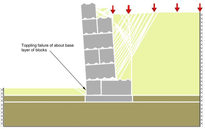
Figure 6.3 Critical failure mechanism for a competent foundation soil
