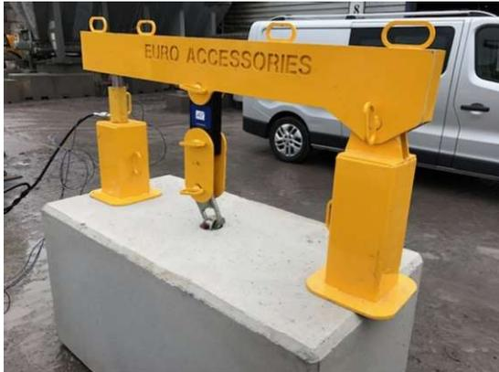
Legato Block at 50% loading of 5.0t Pin Anchor
