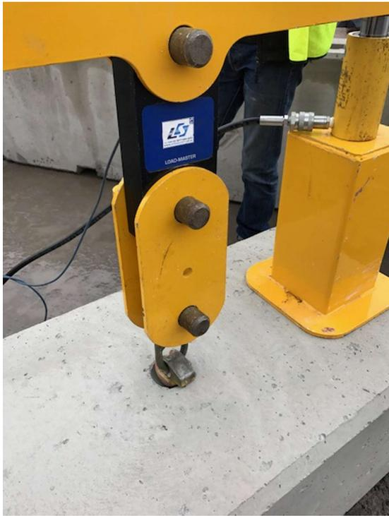
50% Load reading on Duo Block 2.5t Pin Anchor
