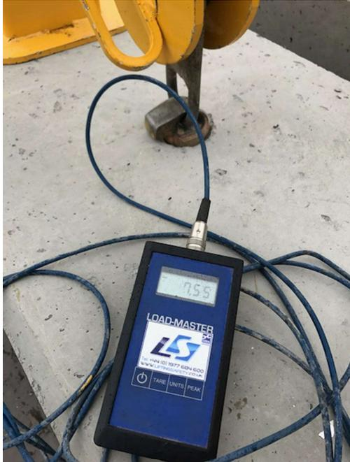
Checking depth of 2.5t Pin Anchor
