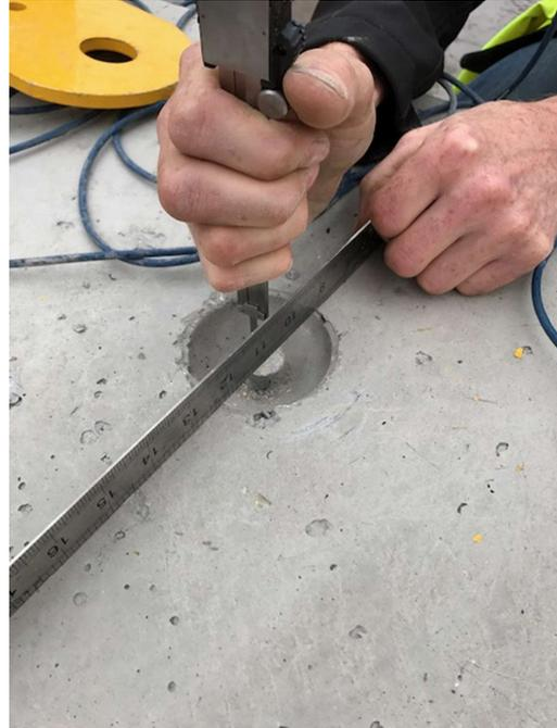
2.5t Pin tested to breaking point in Duo Block showing peak load at 9.3t and clear evidence of the elongation of the pin.
