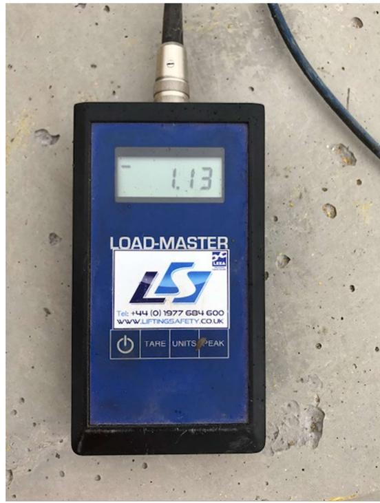
100% load on Duo Block 2.5t Pin Anchor
