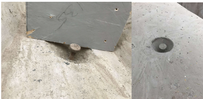
Figure A left hand image with anchor showing clear evidence of creep strain due to repeated use. Right hand image showing anchor set below concrete surface in newly manufactured concrete.
